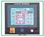
KW's industry-leading Insight® color touch screen HMI is intuitive and self tutoring. Automatic programming eliminates operator error and ensures consistent performance regardless of shift or operator skill. Apache also offers enhanced diagnostics and both networking and remote connectivity options.
