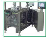
The electrical enclosure is designed to "swing open" to allow total access to the machine interior from either side, improving sanitation and reducing maintenance downtime.
