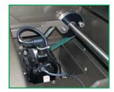
Servo-actuated jaw crank arms are sturdier for longer service life and higher sealing pressure. Maintenance free bearings and guides are all dust tight and long wearing.
